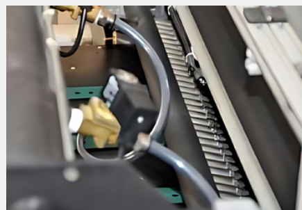
Air-knife Precise Design Suitable For Substrate 130-500gsm Pointed Air-blast On Substrate To Avoid Simple To Set And Ease Of Use
