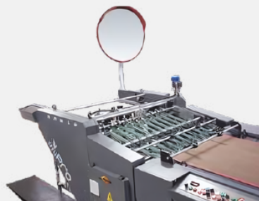
Automatic Stacker Heavy Duty Stacker Pneumatic Joggers Automatic Table Movement Sheet Counter Air-cushening For Thin Paper Stacking
